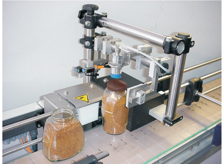
Closure, closure height & metallic foil detection with TSS reject system
