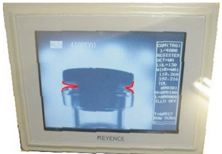
Closure measurement via CCD-camera technology
