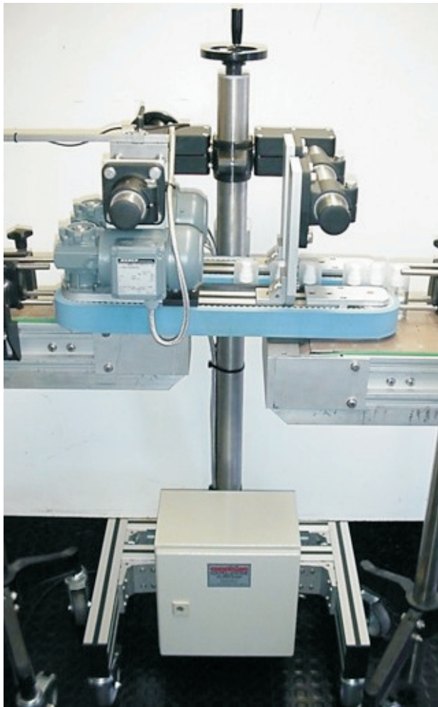
BODE CHEMIE / D - HAMBURG / accumulation conveyor with pneumatic infeed paddel and bottle flow monitoring
