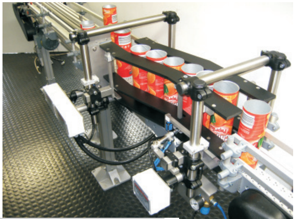
WERZ FLEISCHEREI / D - HEIDELBERG / movable Conveyor with vaccum detector VC 25
