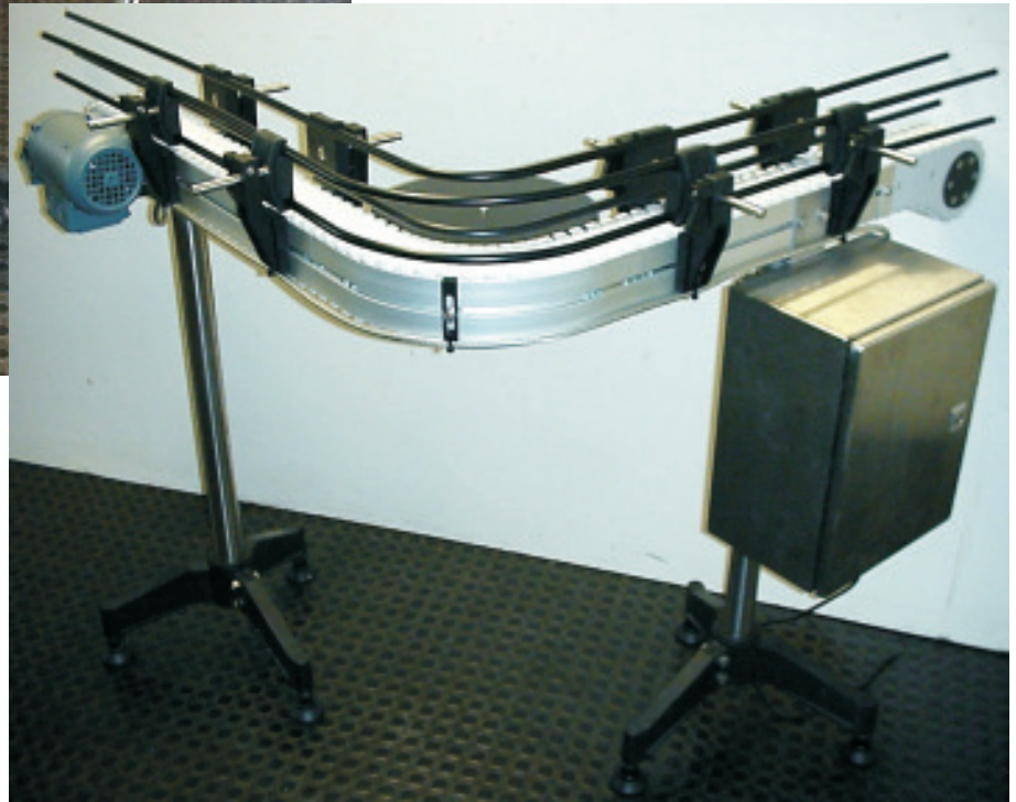
METTLER TOLEDO GARVENS Check Weigher / D - HASEDE / Reject Conveyor with adapter for installation of a return loop conveyor
