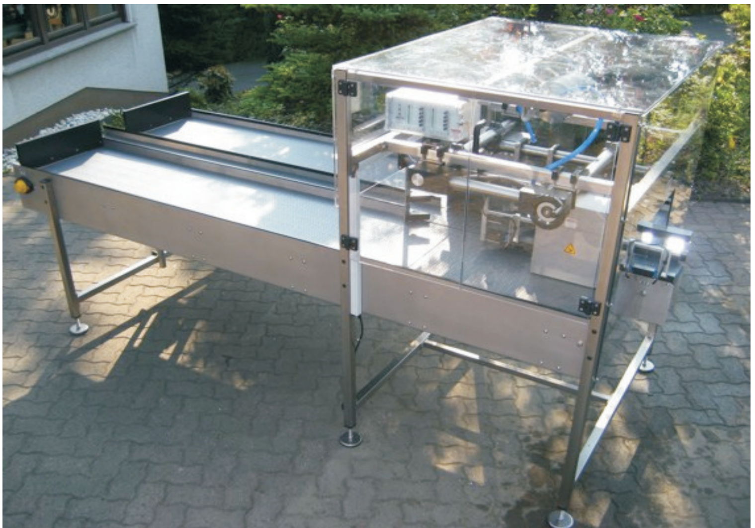
SARTORIUS Check Weigher / D - AACHEN / Conveyor with double reject systems
