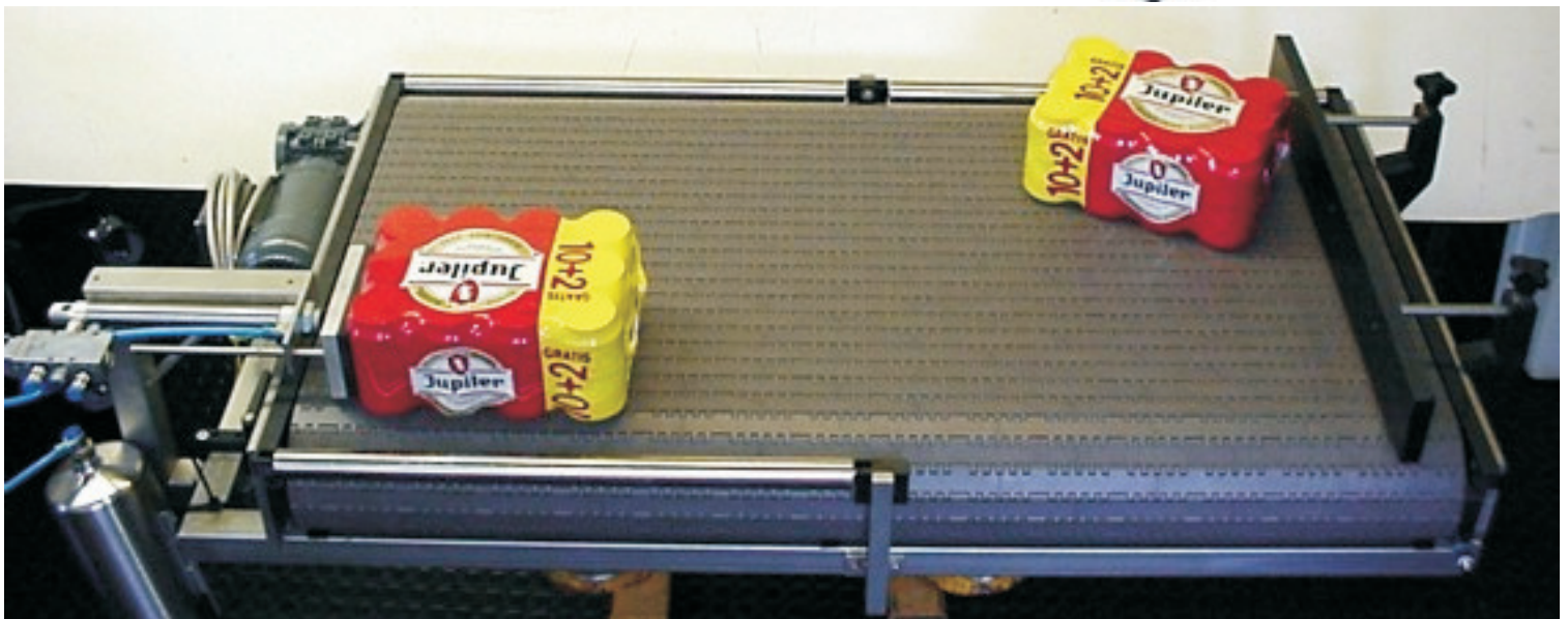
INTERBREW / BE - LEUVEN / 2 pcs. reject conveyor with pneumatic pusher system in 2000mm height
