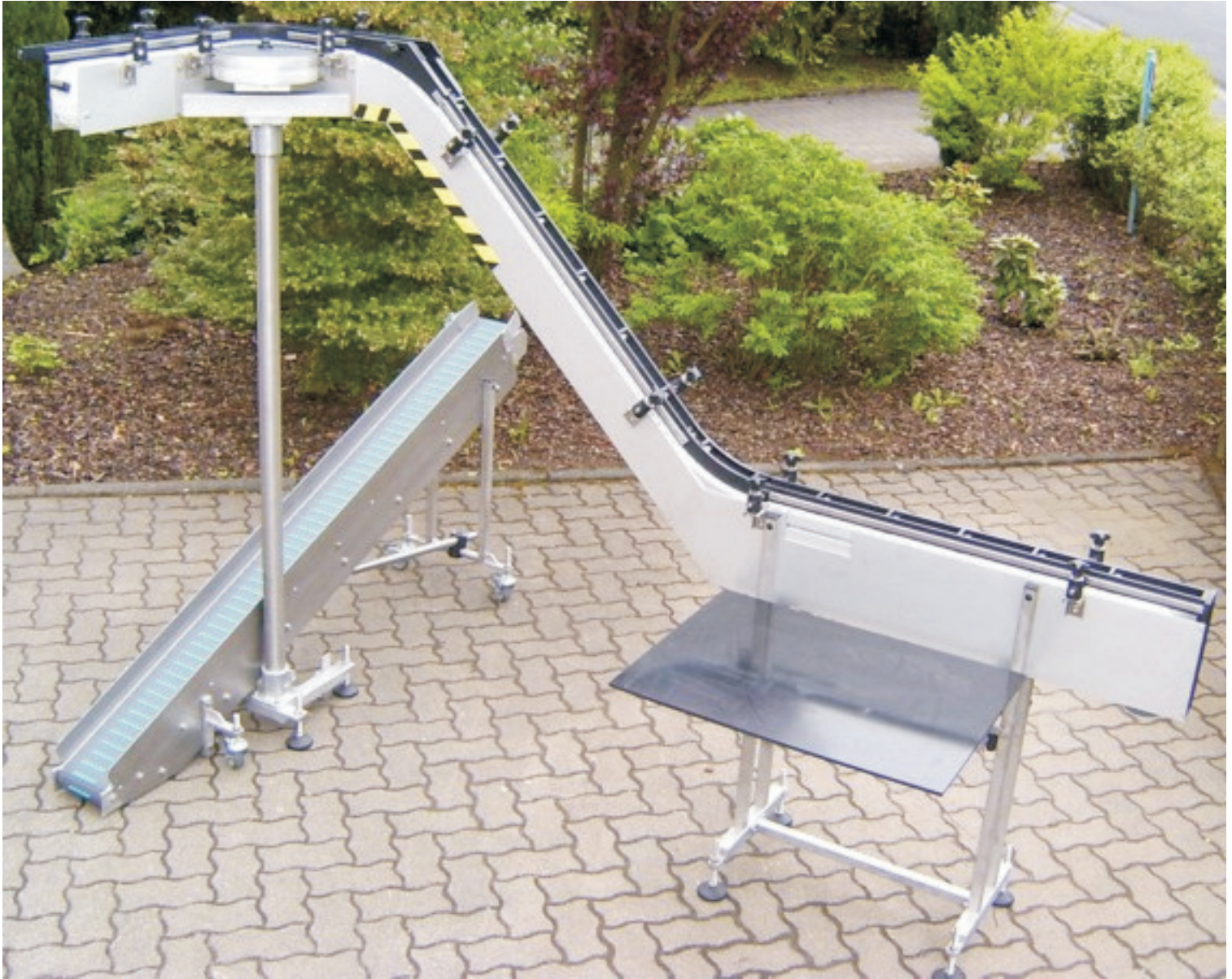
ASELI / D - Berlin / Conveyor for hand packaging in shrink-foil-machine
