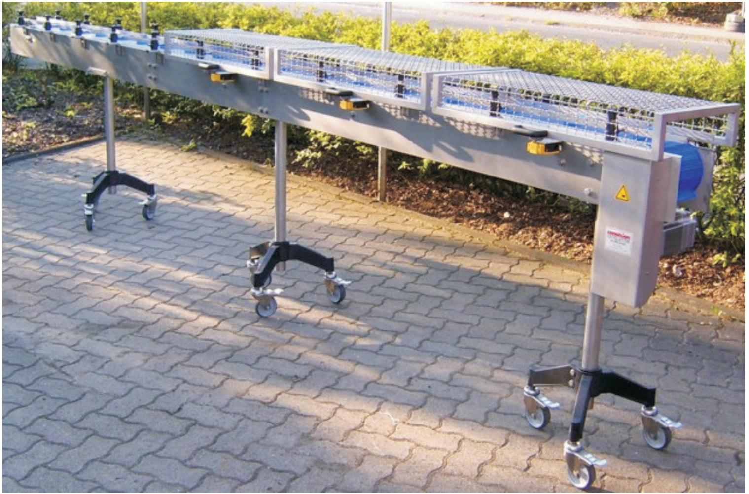
FROSTA FISCH / D - BREMEN / Conveyor for deep frozen fish packs
