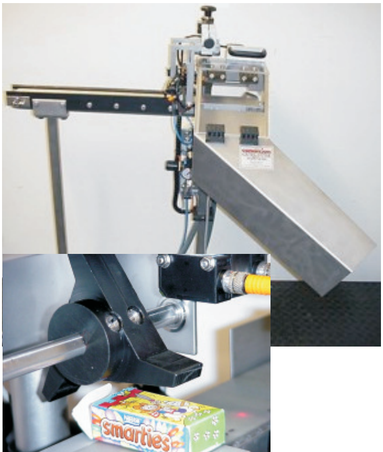
NESTLÉ CHOCOLADE / D - HAMBURG 2 pcs. production conveyor 1000mm installed half inside machine half outside with high speed rejector for small Smarties boxes 800u/min
