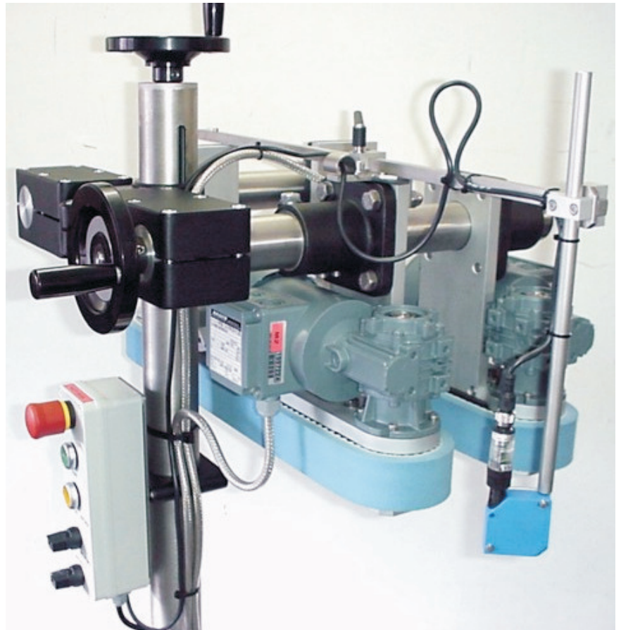
BODE CHEMIE / D - HAMBURG / side-gripper with separate adjustable belts, back-up indicator complete movable on rack
