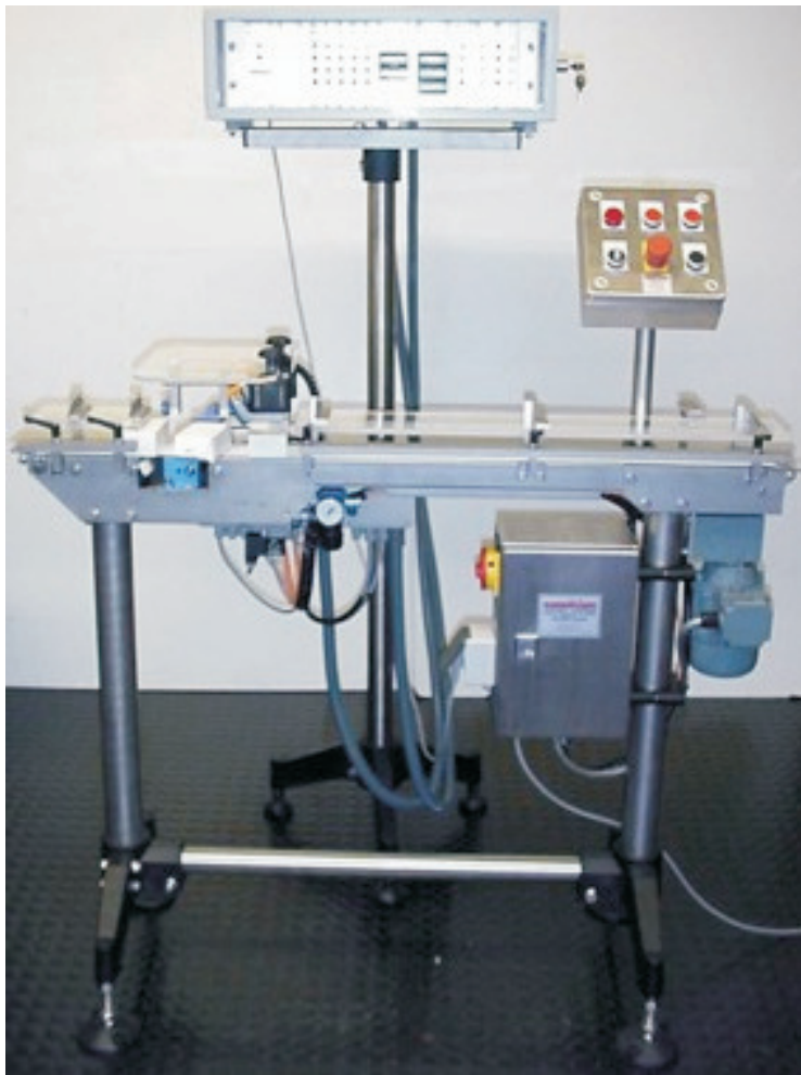
BOEHRINGER - Pharma / D - INGELHEIM reject conveyor with carton box monitoring
