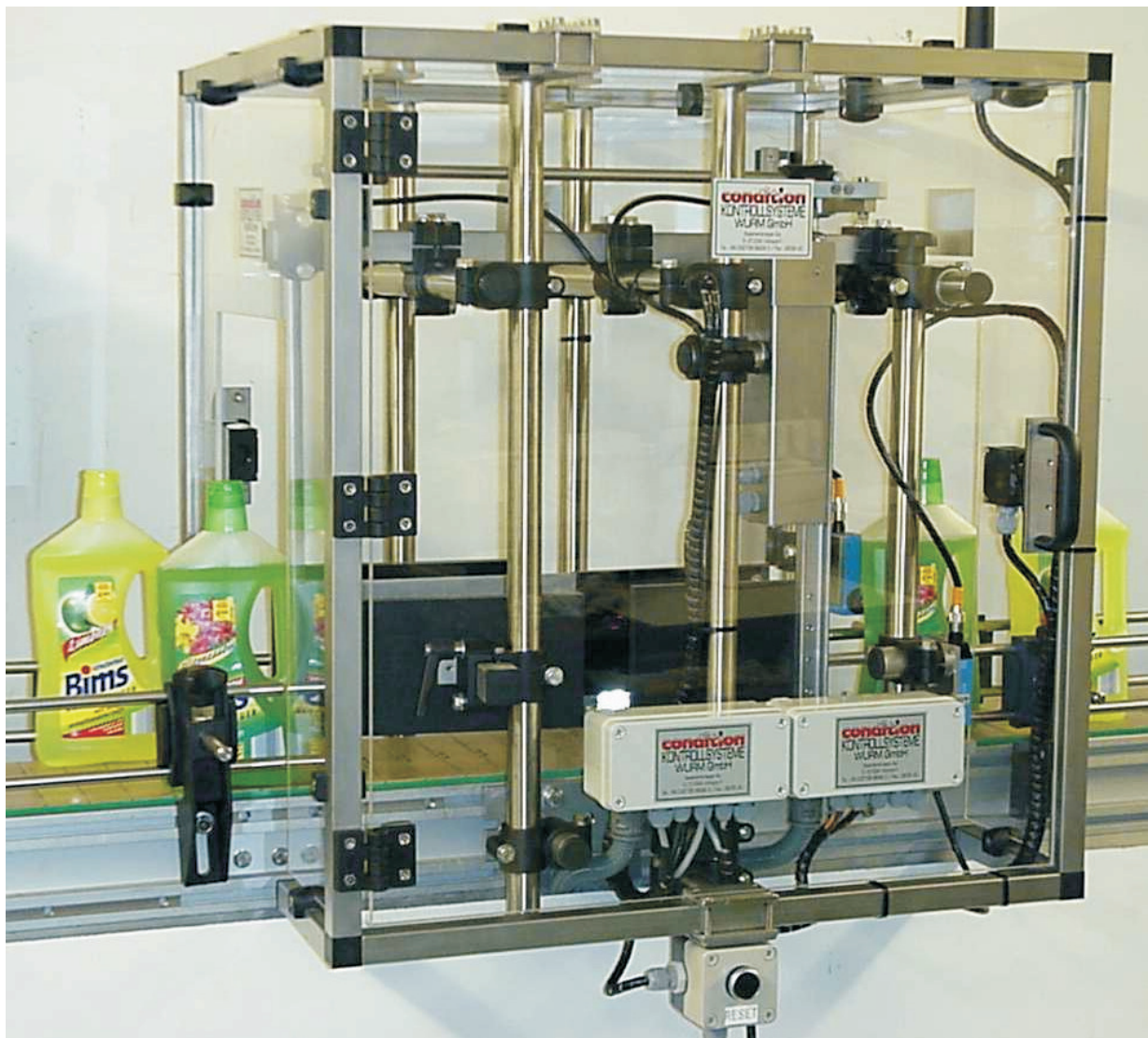
LUHNS GmbH / D - GREVEN / EMW - Reject System with luminescence label detection
