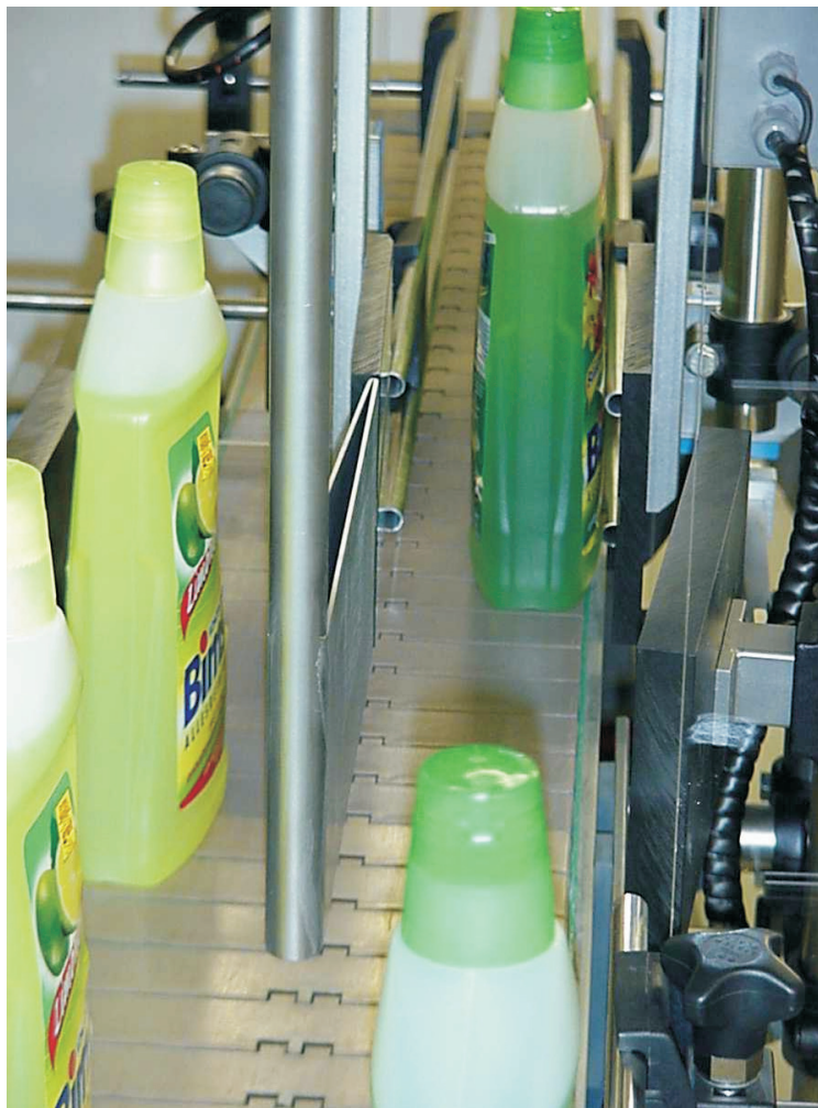
LUHNS GmbH / D - GREVEN / EMW - Reject System with luminescence label detection
