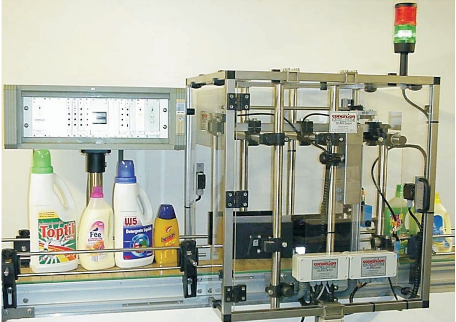
LUHNS GmbH / D - GREVEN / EMW - Reject System with luminescence label detection
